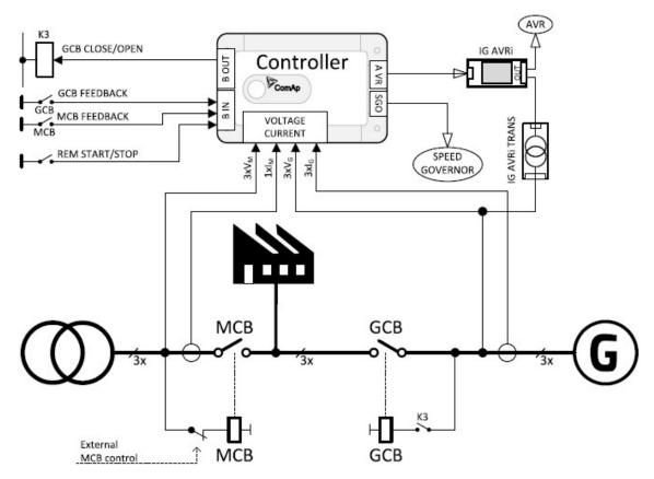
Among other things, it is possible to operate the generator in the stand-alone grid as well as in parallel with the grid.
